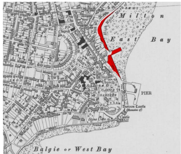
1950 OS Map indicating location of esplanade land reclamation (highlighted in red) and realignment of road network.
